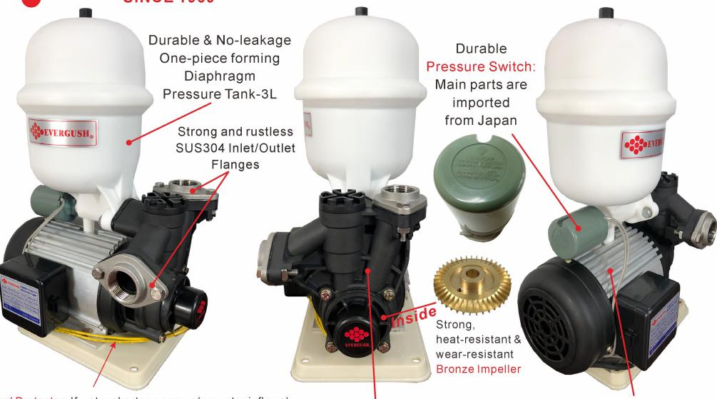
Thermal Protector: If water shortage occurs (no water inflows), the pump is dry-running and causes water temperature rising inside the pump. Once the water temperature reach 65°C, the thermal protector will send a signal to the pump to stop running. To protect motor from burnout due to long-term dry-running.
